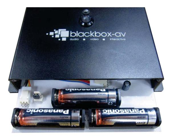
The 3xAA batteries provided with the Visitor Counter should last in excess of 2 years. To change the batteries simply remove the 4 screws at bottom of the Counter and slide the battery plate out.
